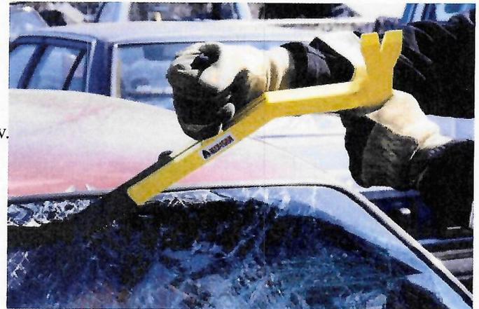
3. Insert blade into opening. Use a swing motion to cut along top and side of windshield. Repeat procedure on other side of windshield.
