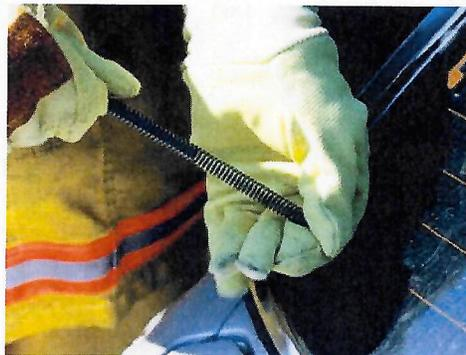
3. Clear edges of frame of any remaining particles of glass.
